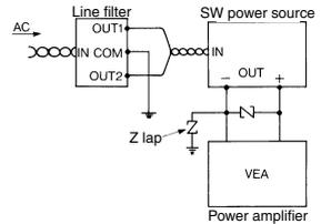
6. If the feed back circuit of the VEA252 will not be used, insert jumper pin J1 on the board on the "1" side. This will disable the feedback circuit, and the VEA252 will assume the same function as that of the VEA251. When inserting the jumper pin J1 in "2" side, activate a feedback signal from the sensor. If the feedback signal is not activated, the current over 1A is output and the valve will not operate even if the externally-set input voltage is changed.
