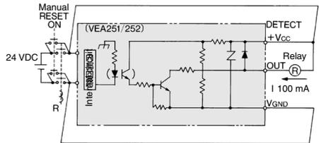
If a short circuit occurs at the current output terminal side, the power supply is shut off immediately to prevent damage to the output circuit of the power amplifier. The manual RESET ON switch is to be pressed to start or restart.
