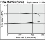
Relief flow characteristics Supply pressure: 0.2 MPa
