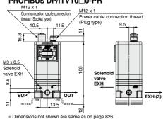
M12 x 1 M12 x 1 Communication cable connection Power cable connection thread thread (Plug type) (Plug type) M3 x 0.5 Solenoid 86 valve EXH Solenoid valve EXH SUP OUT EXH (3) 13.5 ď \* Dimensions not shown are same as on page 826.
