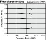
Relief flow characteristics Supply pressure: 0.7 MPa
