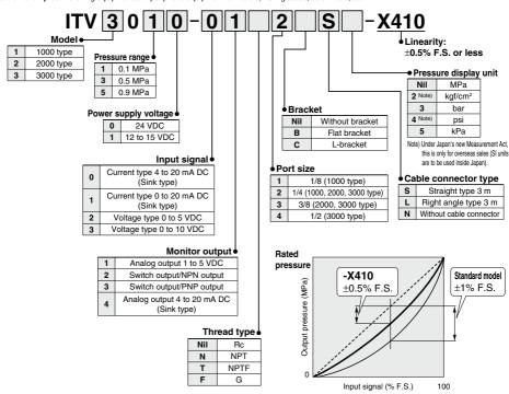
The graph shown above is a typical example. (This graph shows that the output pressure curve is in a negative range when compared to the ideal line.)
