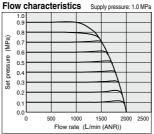
Relief flow characteristics Supply pressure: 1.0 MPa
