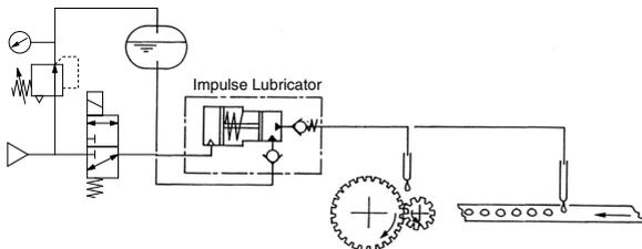
Lubrication to pneumatic equipment such as air cylinders
