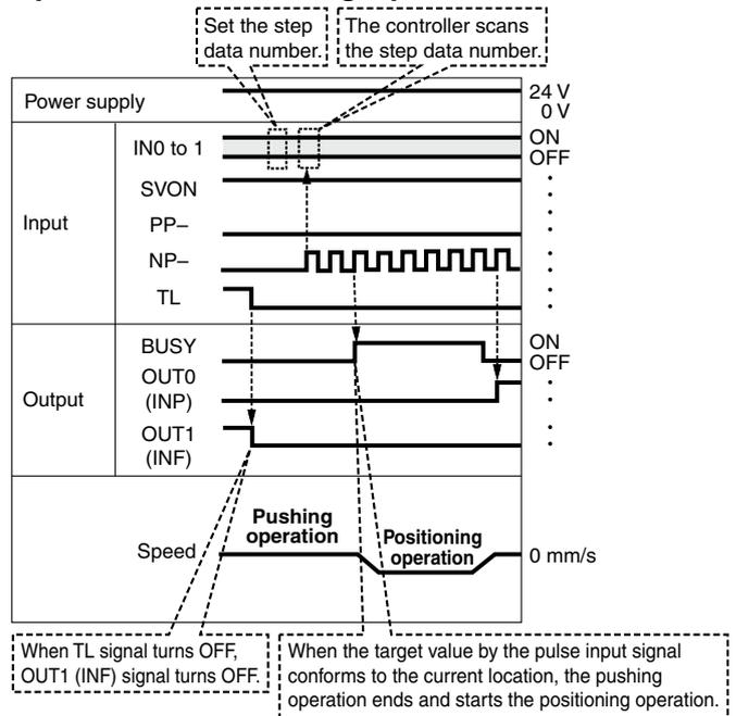
When TL signal turns OFF, OUT1 (INF) signal turns OFF.
