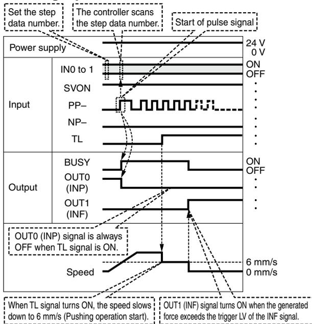
When TL signal turns ON, the speed slows down to 6 mm/s (Pushing operation start).
