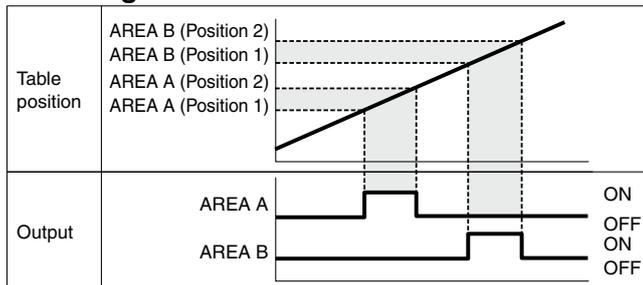
\* Select the AREA signal for the parallel output signal (OUT0 or OUT1).
