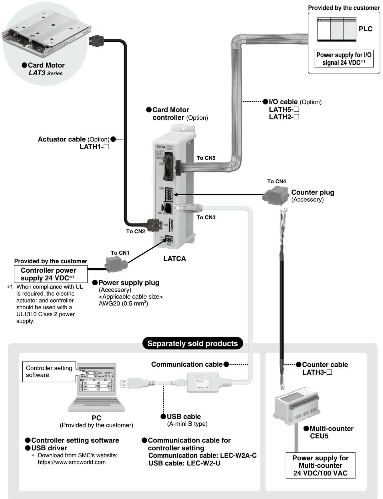
\*1 When compliance with UL is required, the electric actuator and controller should be used with a UL1310 Class 2 power supply.
