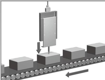
Measurement of glass substrate thickness (multiple points)
