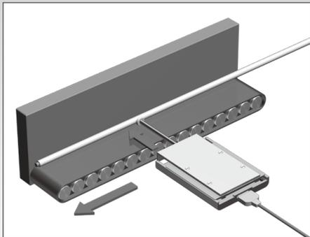
Measurement of tape thickness
