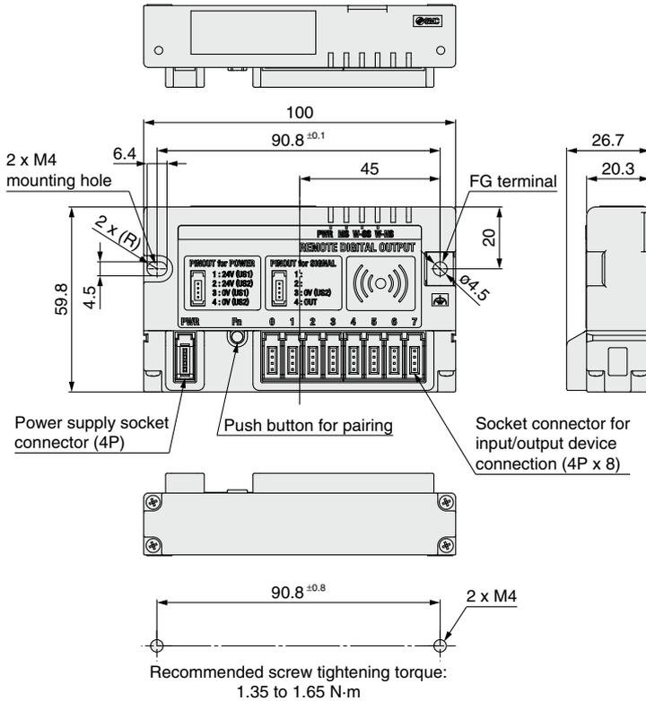
Power supply socket connector (4P)
