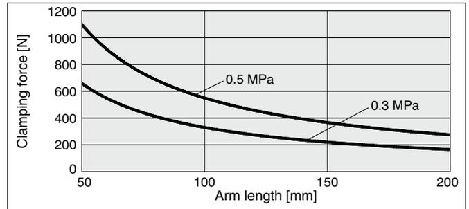
**Calculation example** The maximum clamping force when the arm length is 100 mm and the operating pressure is 0.3 MPa:
