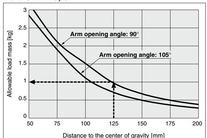
**Calculation example** Arm opening angle: 90°, Distance to the center of gravity L: 125 mm
