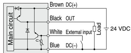
Max. load current: 80 mA, Internal voltage drop: 1.5 V or less
