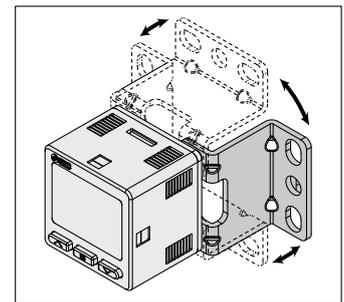
\* Bracket configuration allows for mounting in four orientations.
