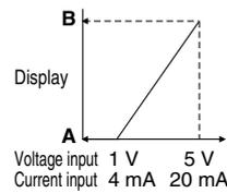
The displayed value to the sensor input can be set as required. (Voltage input: 1 to 5 V/Current input: 4 to 20 mA)
