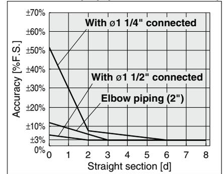
· Do not connect equipment or piping which may generate a fluctuation in the flow or drift at the IN side of the product. When installing a regulator at the IN side of the product, make sure that hunting is not generated.
