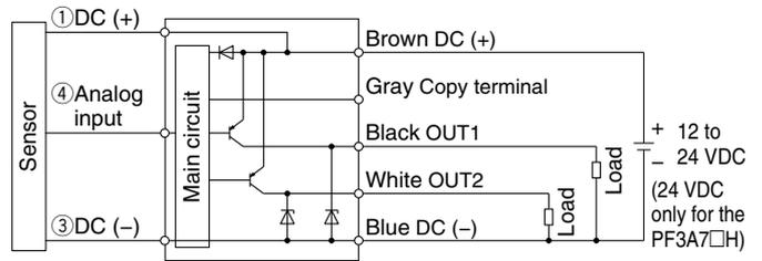
**-RT: NPN (2 outputs) + Analog voltage output**
