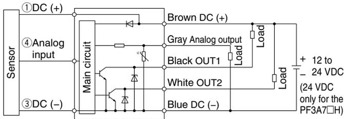
**-RT: PNP (2 outputs) + Analog voltage output**
