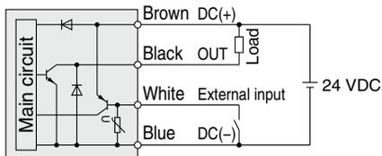
Max. applied voltage: 30 V, Max. load current: 80 mA, Internal voltage drop: 1.5 V or less
