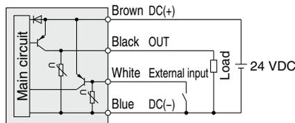
Max. load current: 80 mA, Internal voltage drop: 2 V or less
