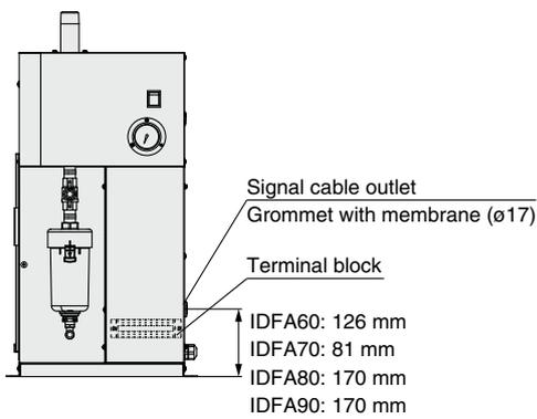
**V** Option symbol**With a timer controlled solenoid valve type auto drain (applicable to moderate pressure)**
