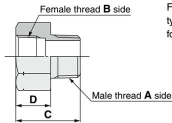
For converting the thread type of an IN/OUT fitting for air dryers.
