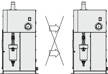
Confirm that the exhaust air does not flow into the neighboring equipment.
