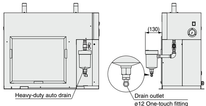
\* The heavy-duty auto drain and piping materials (nipple, elbow) are shipped together with the main body of the air dryer. Customers are required to mount the parts to the air dryer.
