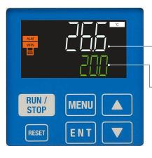
Current value (displayed in white): Discharge temperature, pressure, flow rate, etc.
