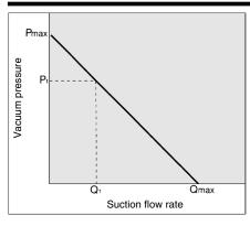
Flow-rate characteristics are expressed in ejector vacuum pressure and suction flow rate. If suction flow rate changes, a change in vacuum pressure will also be expressed. Normally this relationship is expressed in ejector standard use.
