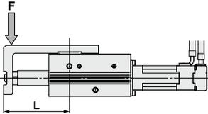
Table displacement due to yaw moment load (marked with the arrow)
