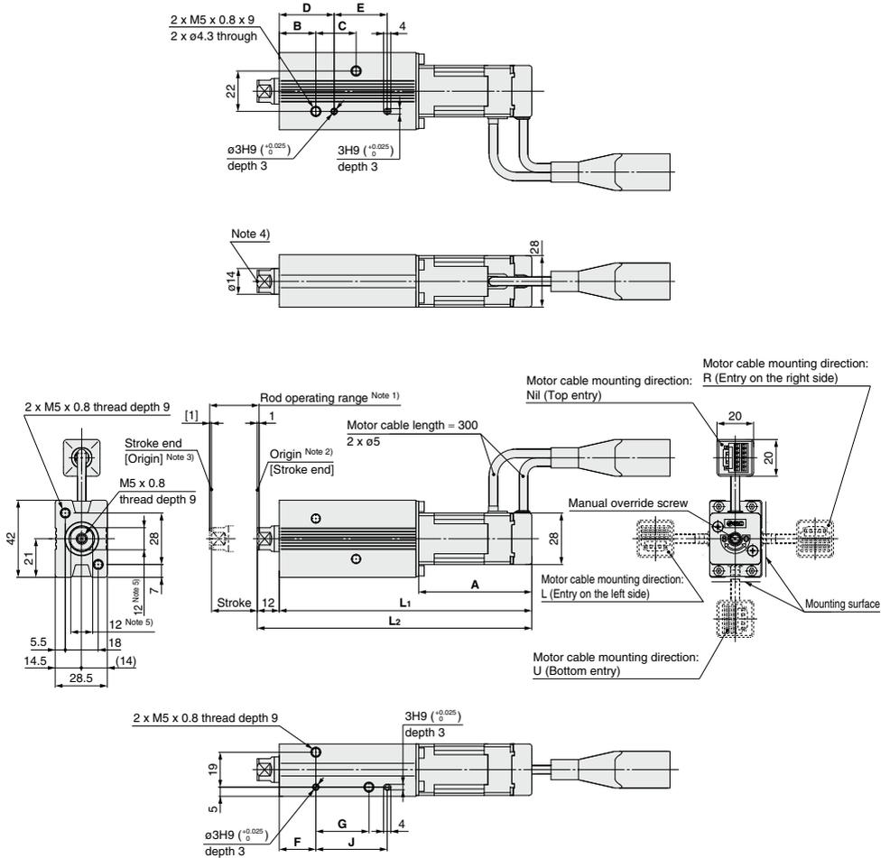
Note 1) Range within which the rod can move when it returns to origin.
