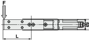
Table displacement due to roll moment load (marked with A)
