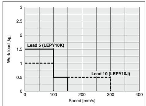
Note) The maximum value of the work load for the positioning operation. An external guide is necessary to support the load. The actual work load and transfer speed change according to the condition of the external guide.
