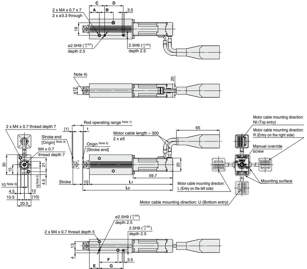
Note 1) Range within which the rod can move when it returns to origin.
