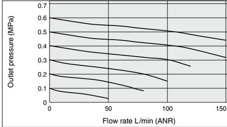
**ARM11AA1-307-1 (One-touch fittings: IN  $\phi$ 6, OUT  $\phi$ 4)** Condition: Inlet pressure 0.5 MPa
