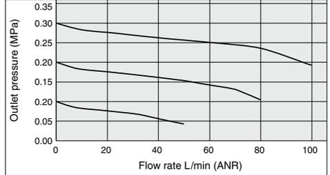
**ARM11BA1-307 (One-touch fittings: IN  $\phi 6$ , OUT  $\phi 4$ )** Condition: Inlet pressure 0.7 MPa
