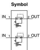
Note) A standard model is equipped with a backflow function. Main valve opens when the inlet pressure is released, and then the outlet pressure backflows into the inlet side.
