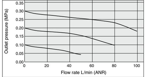
**ARM11BA1-308 (One-touch fittings: IN/OUT  $\phi 6$ )** Condition: Inlet pressure 0.7 MPa
