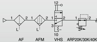
When the air supply is cut off and releasing the inlet pressure to the atmosphere, the residual pressure release of the outlet side can be ensured for a safety purpose.
