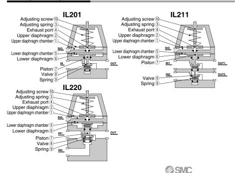
The signal air pressure enters the upper diaphragm chamber 1 to generate a force. When this force is larger than the force generated by compressing the adjusting spring 3, the upper diaphragm 2 is pushed up, the exhaust port 4 is closed, and the signal air pressure enters the lower diaphragm chamber 5 and acts the lower diaphragm 6. This pushes down the piston (7) to open the valve.
