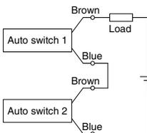
When two auto switches are connected in series, a load may malfunction because the load voltage will decline when in the ON state. The indicator lights will light up when both of the auto switches are in the ON state. Auto switches with load voltage less than 20V cannot be used.
