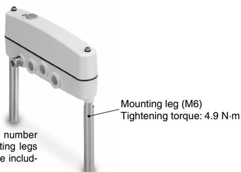
\* When the sub-plate part number (L) is ordered, the mounting legs are not assembled but are included in the same package.
