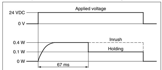
Since the voltage will drop by approx. 0.5 V due to the transistor, pay attention to the allowable voltage fluctuation. (For details, refer to the solenoid specifications of each type of valve.)
