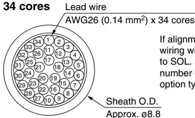
If alignment is not specified, the internal wiring will be double wiring (connected to SOL. a and SOL. b) regardless of number of stations, valve types, and option types.
