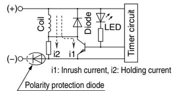
The circuit shown above reduces the power consumption for holding in order to save energy. Refer to the electrical power waveform as shown below.
