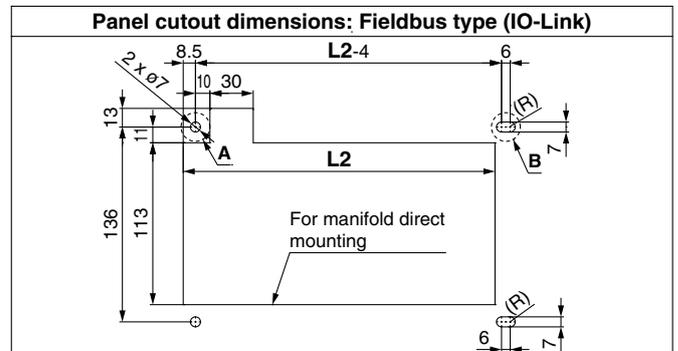
\* When mounting with the mounting leg (L), only the leg mounting holes (round/elongated) are machined.
