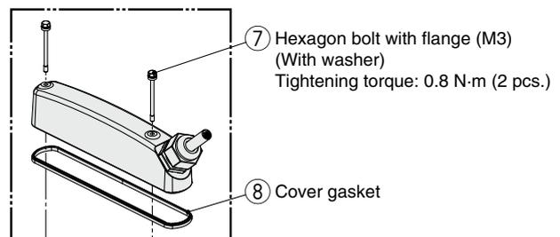
Hexagon bolts with flange and the gasket are mounted.
