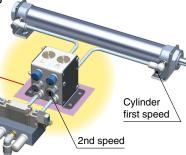
Example of a circuit when performing two-speed control without using DAS
