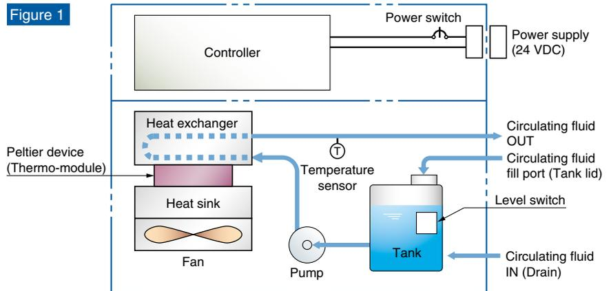
The thermo-con is constructed as shown in Figure 1. The circulating fluid outlet temperature is controlled precisely by a Peltier element (thermo module) between the heat exchanger and heat sink which is controlled by supplying DC power supply. The circulating fluid returns to the tank and is transferred by the pump which is built into the thermo-con, then it goes through the heat exchangers and temperature sensor and out from the circulating fluid outlet.
