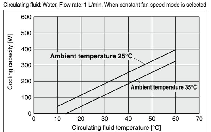
\* For the high-pressure pump (Option), the cooling capacity decreases by approx. 20 W.
