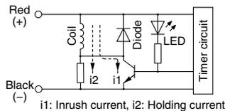
The circuit shown above reduces the power consumption for holding in order to save energy. Refer to the electrical power waveform as shown below.
