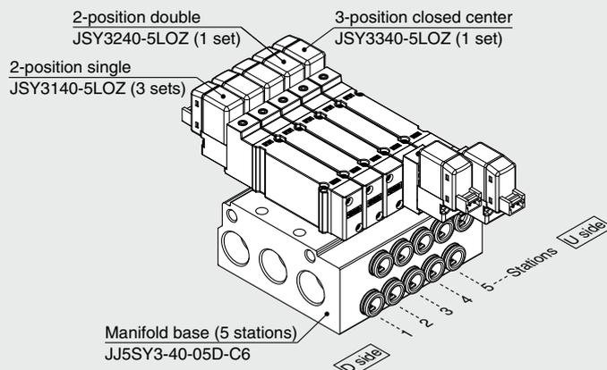
JJ5SY3-40-05D-C6..1 set (Type 40 5-station manifold base part no.)
