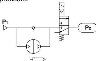
Initially, inlet pressure ( $P_1$ ) passes through the check valve, fills  $P_2$ , and results in  $P_1 = P_2$ .
