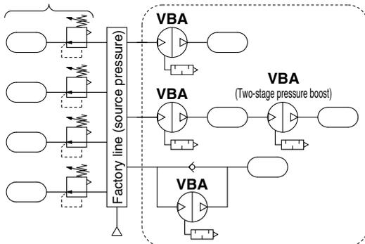
\* When using two booster regulators for 2-stage pressure boost, be sure to supply sufficient flow to each booster regulator in order to stabilize the booster regulator inlet pressure. Refer to Selection 2. on page 10 for the inlet side supply amount.
