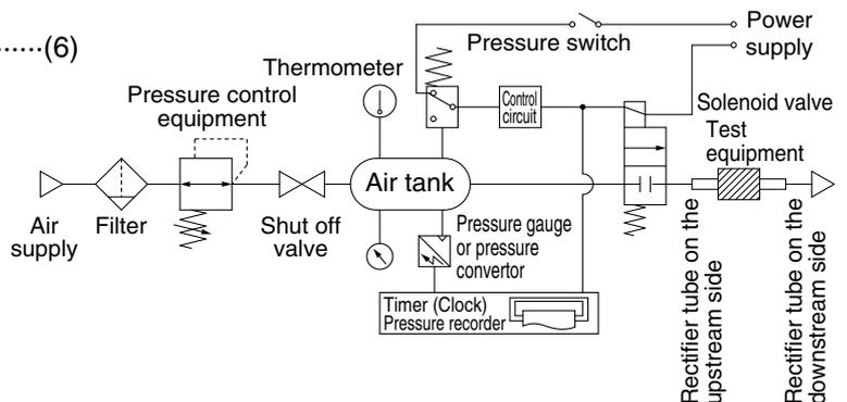
**Fig. (2) Test circuit based on JIS B 8390**
