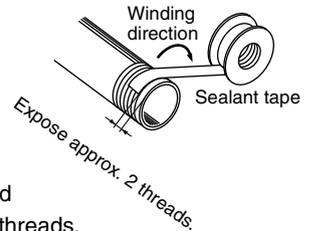
**6. If an excessive amount of thread sealant, such as sealant tape or liquid thread sealant, is used during piping, it will get inside the product and lead to a malfunction.**
