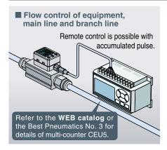
Accumulated indication shows the operating flow rate or residual amount (of N2 etc.) in a gas cylinder.
