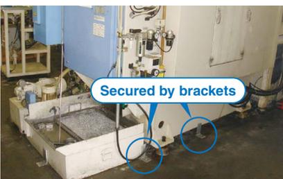
■ Measures to prevent equipment and production materials from falling down
