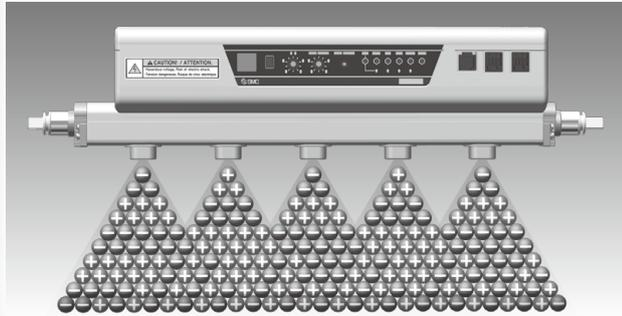
+ ions and - ions are discharged at the same time to allow the + and - ions to reach the workpiece evenly, thereby reducing the potential amplitude.
