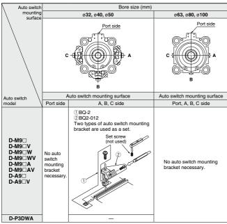
Note 1) For the CDQ2 32 to 50, when a compact auto switch is mounted on the three sides (A, B and C above) other than the port side of bore sizes e32 to e50, the auto switch mounting brackets above are required. Order them separately from cylinders. (It is the same as when mounting compact cylinders with an auto switch mounting rail, but not with a compact auto switch installation groove for the CDQ2LE63 to 100.) Example CDQ2XB32-100DM-M9BW-----1 unit
