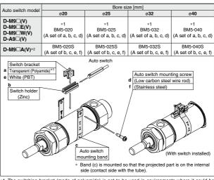
\*1 The switching bracket (made of polyamide) is not to be used in environments where it could be exposed to chemicals (In particular, alcohol, chloroform, methylamine, hydrochloric acid, and sulphuric acid, etc.), as they may affect the performance.
