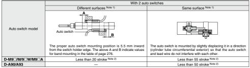
Note 2) Minimum stroke for auto switch mounting in types other than those mentioned in Note 1.
