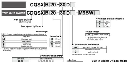
20.25 5, 10, 15, 20, 25, 30, 35, 40, 45, 50 · Manufacturing of intermediate stroke
