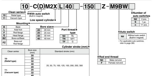
\* Manufacture of intermediate strokes in 1 mm increments is possible. (Spacers are not used.)
