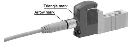
Note) When installing a connector cable, directions must be confirmed. When installing SMC's connector cable (V100-49-1□), align the arrow mark of the connector and the triangle mark of the valve. Twisting without alignment may damage pins and cause malfunction.
