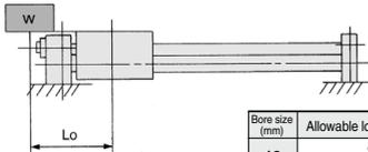
Lo: Distance from center of slide block to load center of gravity (cm)
