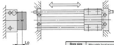
Lo: Distance from mounting surface to load center of gravity (cm)
