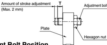
**Adjustment Bolt Position (at the time of shipment), Hexagon Nut Tightening Torque**
