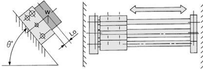
Lo: Distance from mounting surface to load center of gravity (cm)
