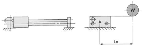
Lo: Distance from mounting surface to load center of gravity (cm)
