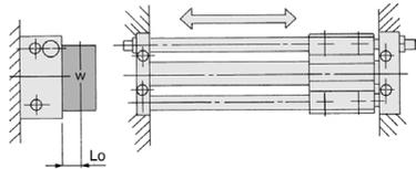
Lo: Distance from mounting surface to load center of gravity (cm)
