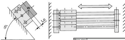
Lo: Distance from mounting surface to load center of gravity (cm)
