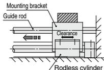
Shaft alignment variations are offset by providing clearance between the mounting bracket and cylinder. Moreover, the mounting bracket is extended above the cylinder shaft center, so that the cylinder is not subjected to moment.
