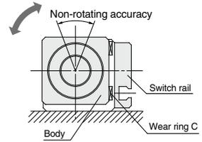
Note 1) Avoid operations where rotational torque (moment) is applied. In such a case, the use of an external guide is recommended.
