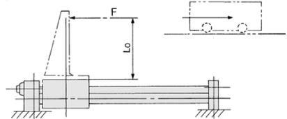
F: Drive (from slide block to position Lo) resistance force (kg)
