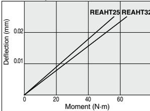
**Displacement of Table due to Roll Moment Load**
