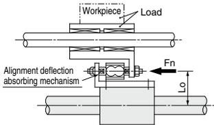
**<Data (A): Distance from Cylinder Shaft Center — Allowable Driving Force>**
