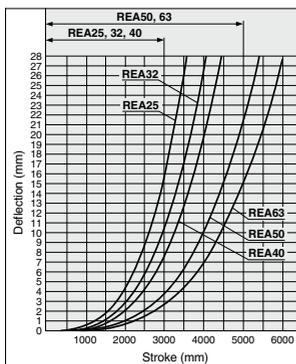
\* The above deflection data indicate values for external movement within the stroke.
