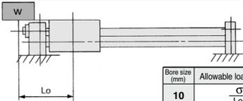
Lo: Distance from center of slide block to load's center of gravity (cm)
