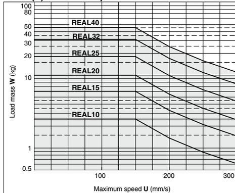
**Examples of Allowable Load Mass Calculation Based on Cylinder Mounting Orientation**
