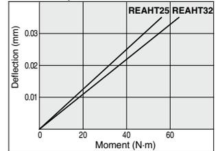
Note) Deflection when a moment other than the above is applied can be specified by extending the lines in the graphs above.
