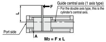
Note) Deflection: Displacement of section A when force acts on section F
