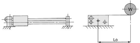
Lo: Distance from center of side block to load's center of gravity (cm)
