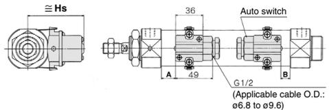
**Auto Switch Proper Mounting Position (Detection at Stroke End) and Its Mounting Height**
