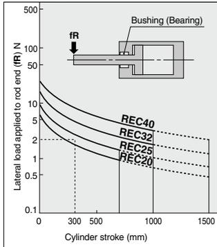
\* The above curve in the graph refers to P = 0.5 MPa of supply pressure. If supply pressure is other than P = 0.5 MPa, please figure out a max. stroke, using proportional calculation.
