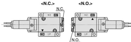
1. Remove the body from the sub-plate and reset the "▼" mark on the body corresponding to the "N.O." mark on the sub-plate as shown in the figure above.
