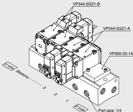
VV3P3-41-051-02 ..... 1 set (Type 41, 5-station manifold base part no.)
