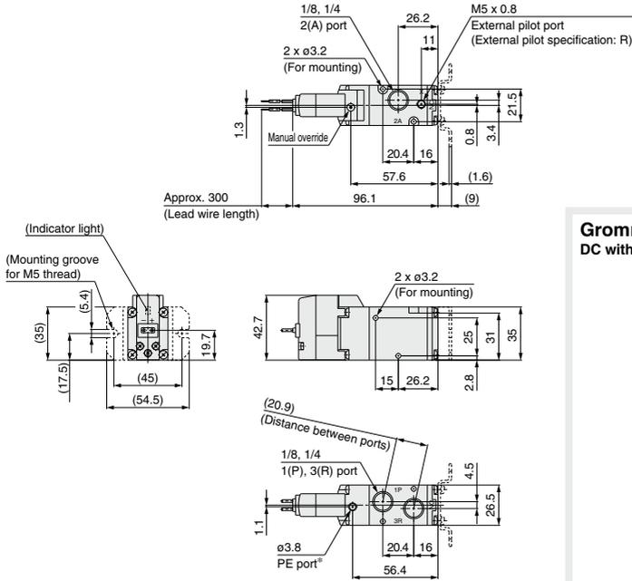
\* Refer to page 1291 separately when piping to PE port is required.
