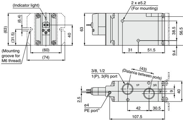
\* Refer to page 1291 separately when piping to PE port is required.
