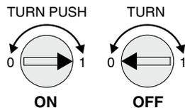
It can be locked in the ON state by turning the manual override to the right, setting the ► mark to 1 and pushing it.
