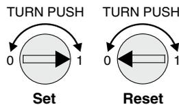
It can be locked in the set state (flow: P → A) by turning the manual override to the right, setting the ► mark to 1 and pushing it.
