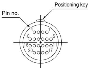
Circular connector pin arrangement
