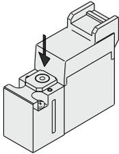
It is turned ON by pushing the button in the direction indicated by the arrow until it hits the end and turned OFF by releasing the button.
