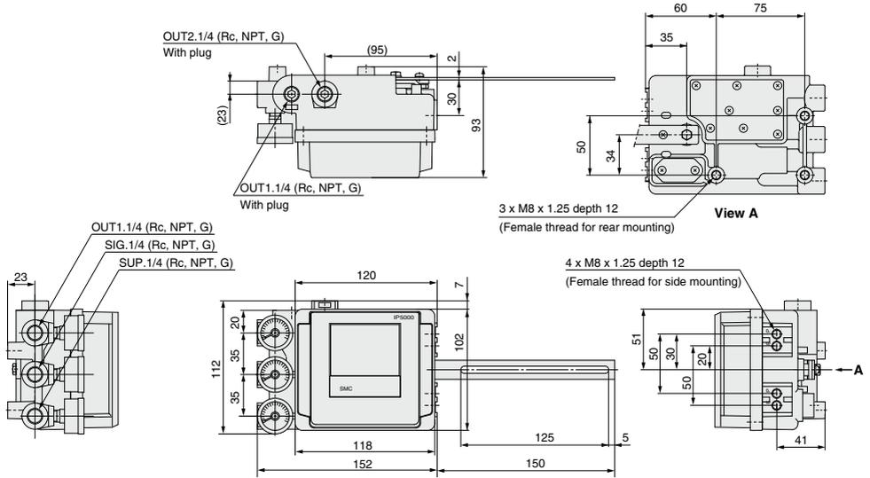
**IP5100 type (Rotary type cam feedback)**
