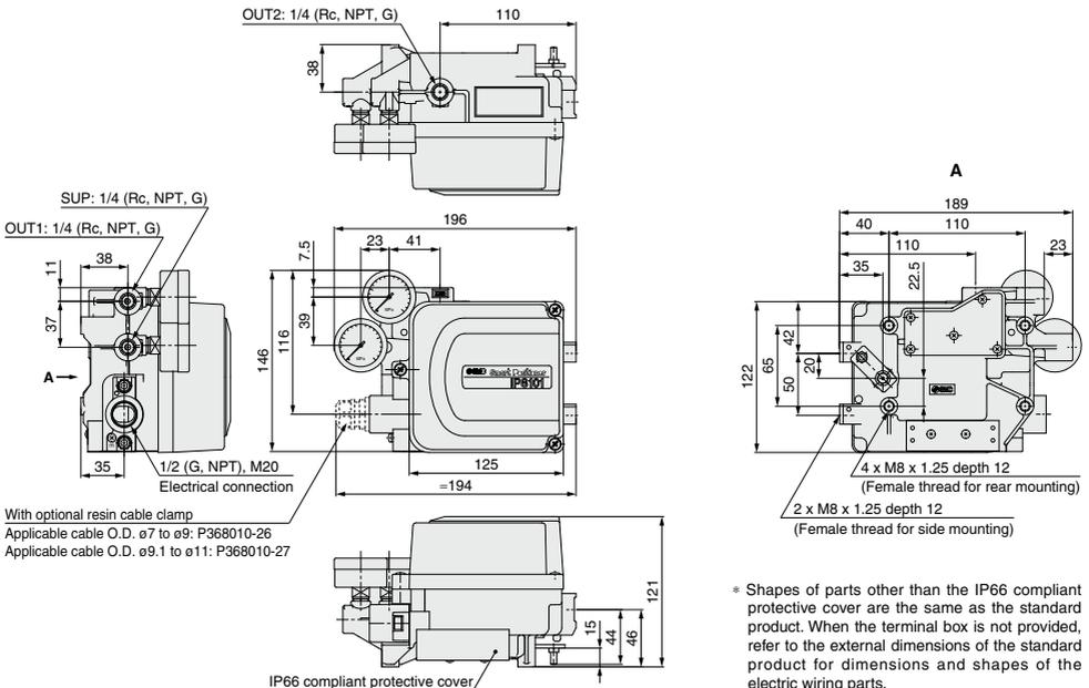
\* Shapes of parts other than the IP66 compliant protective cover are the same as the standard product. When the terminal box is not provided, refer to the external dimensions of the standard product for dimensions and shapes of the electric wiring parts.
