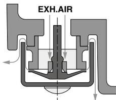
A centralized exhaust system employs the combination of the check valve and the labyrinth effect enhancing both dustproof and waterproof performance.
