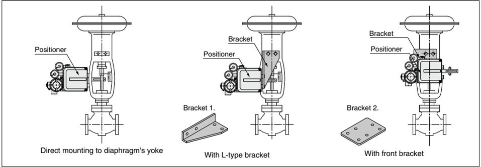
2. The feedback lever that detects the displacement of valve stems should be mounted at a position so that the lever is at right angles to the valve stem for an input current of 50%. The figure is the configuration viewed from the front.
