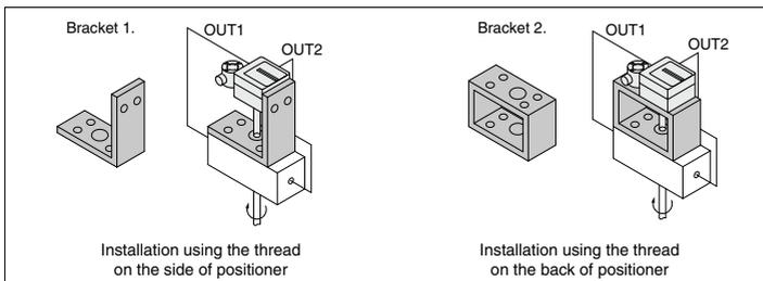
Installation using the thread on the side of positioner
