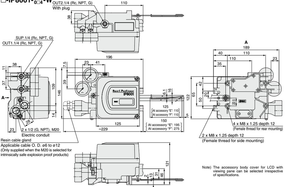
Note) The accessory body cover for LCD with viewing pane can be selected irrespective of specifications.
