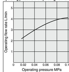
Conditions: 1. Lifting range 1 m. 2. Collection tube (T0645) length
