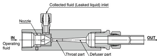
When the operating fluid is flown from the IN side (nozzle, throat part, defuser part) at a certain flow rate or more, the negative pressure is generated in the throat part. This negative pressure is used to suck up the leaked liquid and discharge it together with the operating fluid toward the OUT side to return it to the tank.
