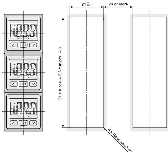
Note) When providing a curvature radius (R), keep it to R2 or smaller.
