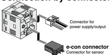
Connector for power supply/output
