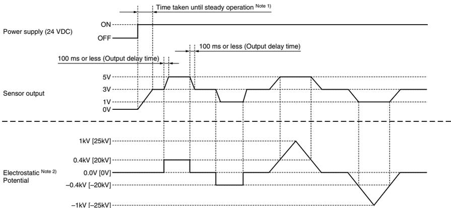
Note 1) The sensor is ready for operation approximately one second after power-on but may provide unsteady readings. It is therefore recommended that the sensor be used more than 10 minutes after power-on.
