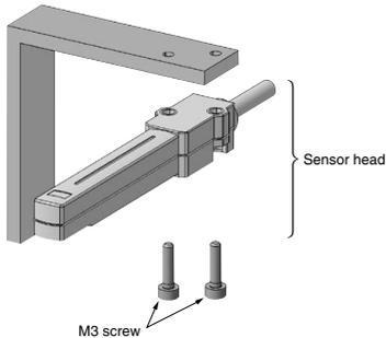
4. Align bolts with their seating surfaces to mount the sensor head. Mounting it by inserting the bolts from the opposite side may damage the sensor head.
