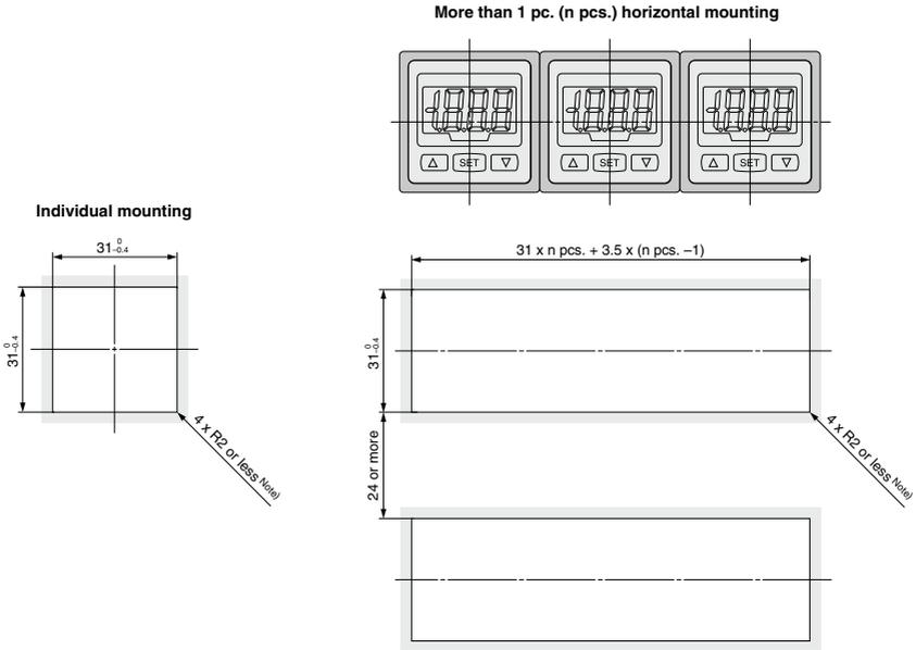
Note) When providing a curvature radius (R), keep it to R2 or smaller.
