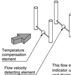
This flow switch uses L/min as the flow rate indicator unit. The mass flow is converted and displayed under the conditions of 0°C and 101.3 kPa and 20°C and 101.3 kPa.
