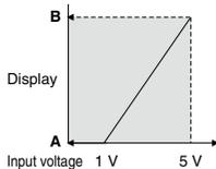
The sensor input range can be set to the required value and displayed. (Voltage input: 1 to 5 V)
